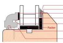
Arbosil silicone Security Glazing Tape 2 x 8mm glazing tape compressed to 1.5mm Friction fit between uPVC clip and timber composite bead Surface connection, to match clip with bead
