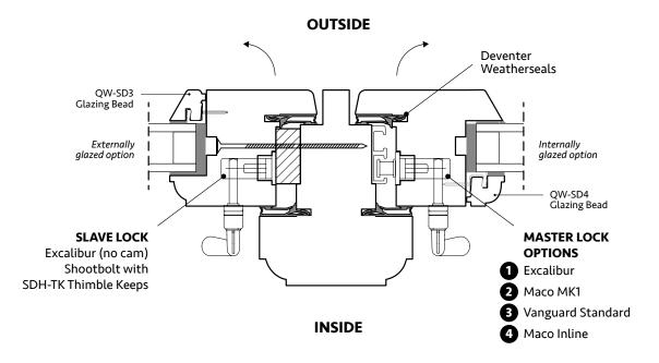
You could use the claw version of the Excalibur shootbolt system, with stormproof keeps fixed to the surface of the flying mullion. Other options include the Maco MK1, Maco Inline, or the Vanguard Standard. In the section drawing above there are suggestions for other products we recommend when producing this type of window.
