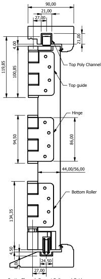
SectionThrough Door at Roller and Guide
