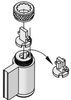
5 Test the key operation. If the key is difficult to insert or tight when turning, then the cap maybe too tight. Loosen the cap one notch at a time and try the key again. If the key inserts and turns OK, but is difficult to remove, then the cap may be too loose. Tighten up the cap one notch at a time. Adjust the cap until the key inserts, turns and removes easily.
