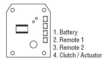
**REM 1** is intended for use when there is a need to allow a visitor to open the door after having been identified by intercom or by sight from within. **REM 1** would be connected to a pushbutton on a reception desk, or to the appropriate button on an intercom. Pushing the button would cause the Blue LED to light and would release the lock for the normal set time.
