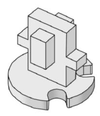
**Classroom Function** tailpiece allows key to turn 90° clockwise and be removed leaving the handle engaged in Code Free Mode. Code Free Mode is cancelled by turning key 90° anti-clockwise.
