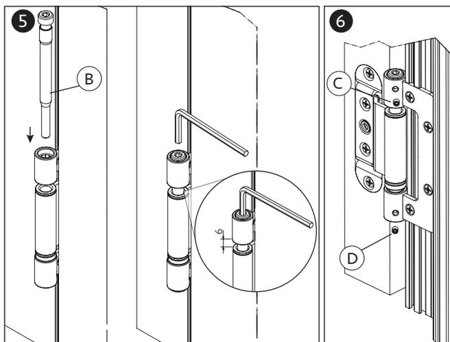
Insert the sash into the frame and screw in the pin marked B with a 4 mm Allen Key till the measure 6mm is reached.
