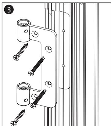
Fasten the frame part with fasteners suitable for the material of your door or window.
