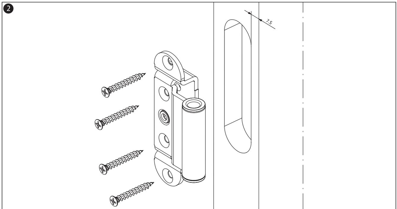
Fasten the sash part into the milling with fasteners suitable for the material of your door or window.
