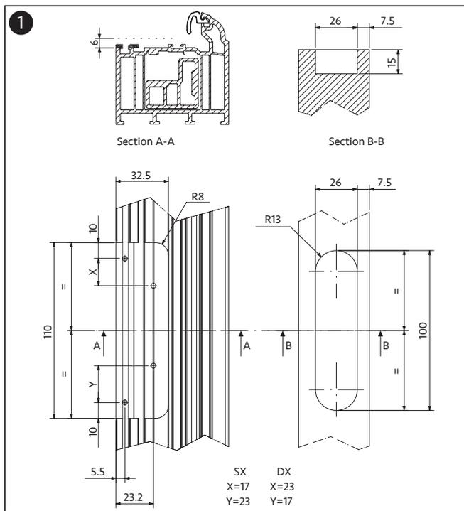
Please verify that the space within your door or window allows the fitting of the hinge as shown in the diagram.
