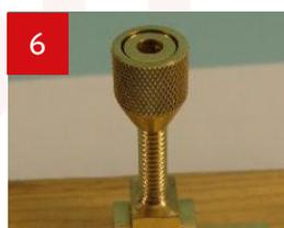
6 This is how the Fastener will look when the Cap is locked and the Collar is up tight to the back of the Cap.
