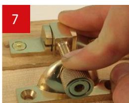
7 Push the Arm of the Fastener down, place the Keep tight up behind the Collar, so the Collar fits snug into the U of the Keep, making sure the Keep is in a central position and square to the Arm.
