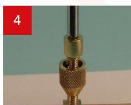
4 Move the Collar down the Arm of the Fastener for the moment and tighten the Lockable Cap until the key will not turn anymore (make sure you do not over tighten or you may damage the Cap).
