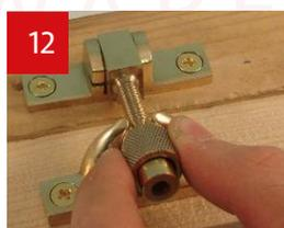
12 Un-tighten the Collar, this will now allow the Arm to come out of the U of the Keep to swing open.
