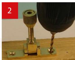
2 Drill out the pilot hole, remove any sawdust.
