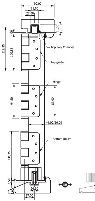
SectionThrough Door at Roller and Guide
