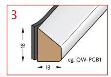
Apply 2.0 mm double sided glazing tape to glazing face of bead.
