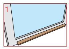
Cut beads to required lengths, recommend to cut top to bottom rails square and scribe the side rails.
