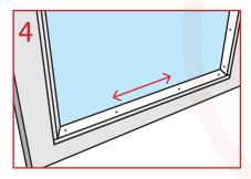
Pin beads every 150 mm to 200 mm securely to frame. Pin on end of each bead for extra security.
