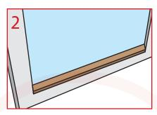
Check beads fit correctly in window frame.
