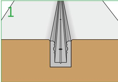
Fit clip (QW-SC1) into groove and secure using pins/staples or glue (test for secure fixing).
