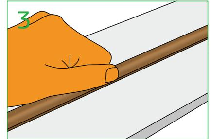
Clip parting bead(QW-CPB8) and/ or staff bead (QW-CSB20) into the fitted clip (QW-SC1) push or tap down until you hear the click.
