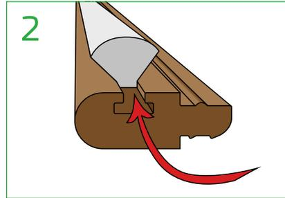
Slide seal (supplied separately) into pre-prepared parting (QW-CPB8) and/ or staff (QW-CSB20) bead.
