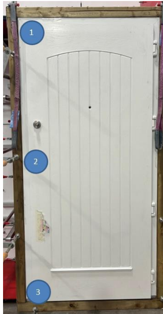
Figure 2 – Position of deflection measurement sensors
