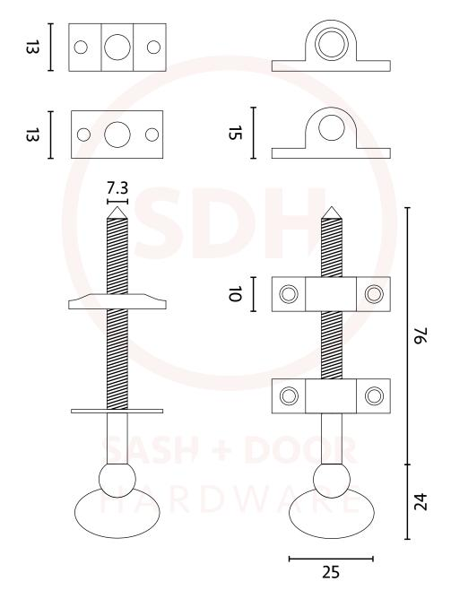
NOTE : This product is made from Cast Brass and manufactured using the Traditional Sand Cast method. The items requiring a Lacquer protection are protected using the Electrophoretically Lacquered process giving a very attractive long-lasting product.
