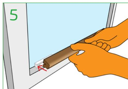
Starting with the base bead, peel off the protective paper strip from the dry glaze tape and push-fit the bead onto the clips along the base. Use a soft faced mallet to tap bead into position, an audible "click" will signal correct fitting.
