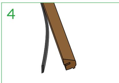
Apply strip of self-adhesive dry glaze tape to back edge of QW-GB5A (SD1A) bead. The tape should be at least 2.5 mm thick to ensure adequate compressive bond.
