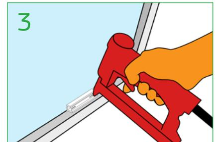
The clips can be fixed using staples, screws or pins. We recommend to use 2 x 80 series staples 12 mm (or longer if preferred) per clip. With the air gun regulators set at approx. 4 bar. Ensure fixings do not protrude into the clip channel and foul bead fittings.
