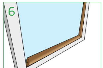
Repeat the process for the jambs and top. The beads will sit automatically in line with frame and should not protrude when pushed correctly onto the clips.
