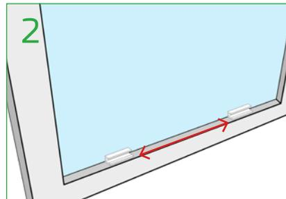
Ideal clip length is 50 mm and 75 mm (but longer length can be used if required). We recommend clips should be spaced at 150 mm intervals. This is a customer preference – the more clips the stronger the fixing.
