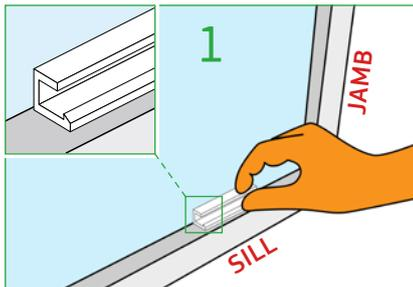
Fit glass panel safely into the frame as required. Offer clip QW-GCA to frame against glass ensuring the correct orientation.
