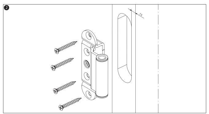
Fasten the sash part into the milling with fasteners suitable for the material of your door or window.
