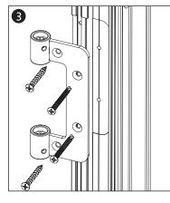
Fasten the frame part with fasteners suitable for the material of your door or window.
