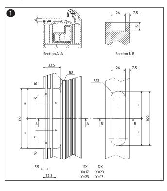
Please verify that the space within your door or window allows the fitting of the hinge as shown in the diagram.
