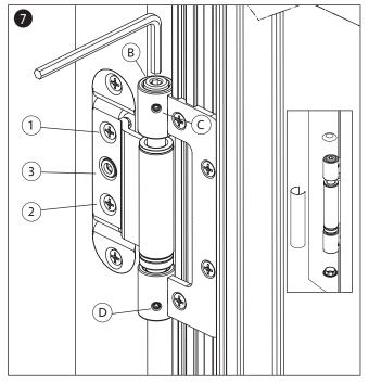
Insert the sash into the frame and screw in the pin marked B with a 4 mm Allen Key till the measure 6mm is reached.
