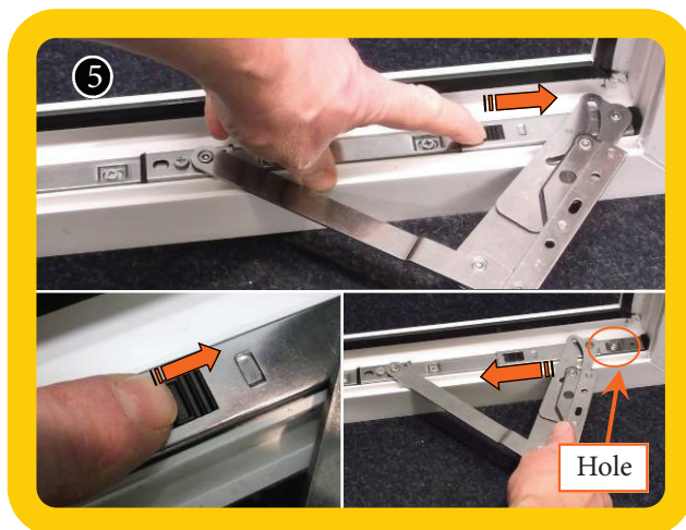
Slide "Easy Clean" activation button and move Top Slider until final screw position is exposed and insert screw
