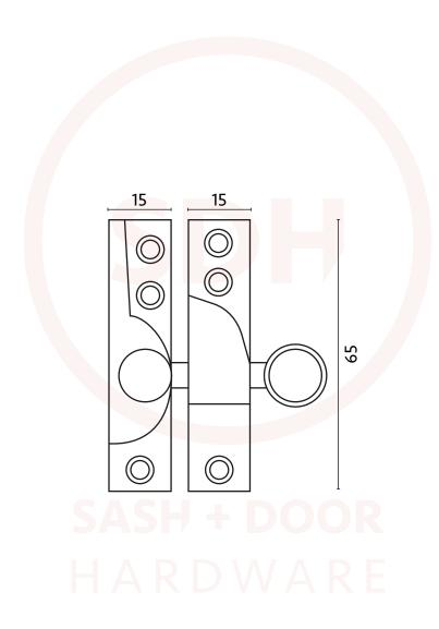
NOTE: This product is made from Cast Brass and manufactured using the Traditional Sand Cast method.
