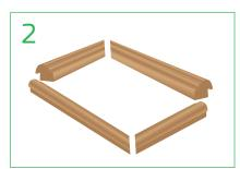
Measure and mitre cut the bead to suit the panel cut out.
