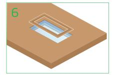
Apply high strength, waterproof timber adhesive to door groove and/or base of cassette, subject to adhesive manufacturers recommendations. Assemble cassette into door groove, apply pressure and allow to cure. Use panel pin fixings for added security.
